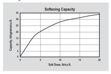
SOFTENING CAPACITY — Capacity is based on 2:1 Ca:Mg ratio, 500 ppm TDS as CaCO3, 0.2% hardness in the salt, and 10% brine concentration applied co-currently through the resin over 30 minutes. No engineering downgrade has been applied.
